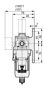
\*1. Dimensions when the digital pressure sensor is assembled.
